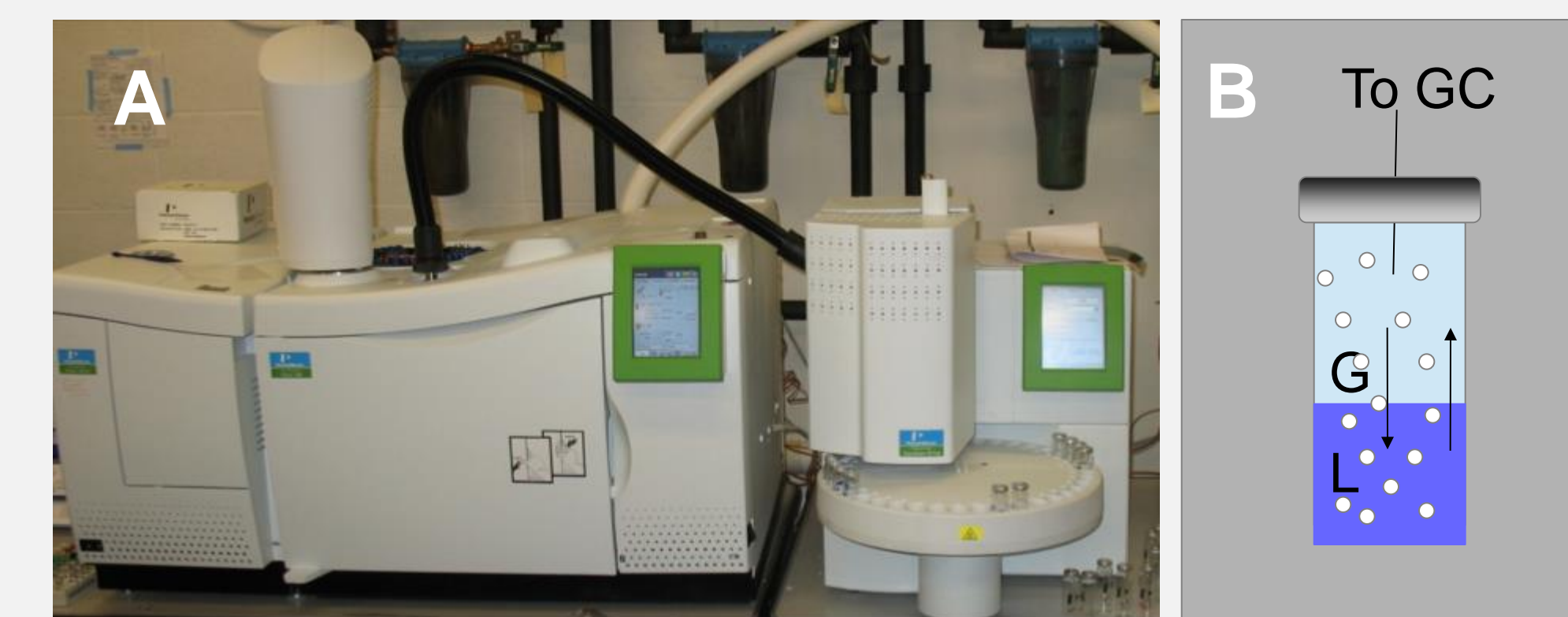
Figure 5. A) Image of PerkinElmer ClarusGC with headspace autosampler. B) Diagram of headspace mechanism
